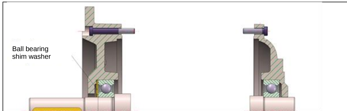
Fig. 1: Constructional design of bearings sizes 63-112
