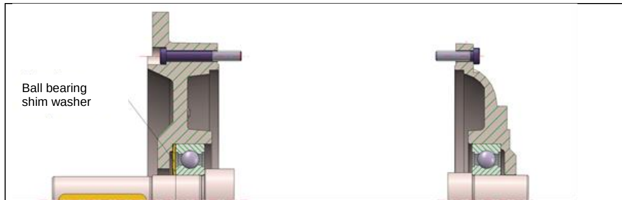
Fig. 1: Constructional design of bearings sizes 63-112
