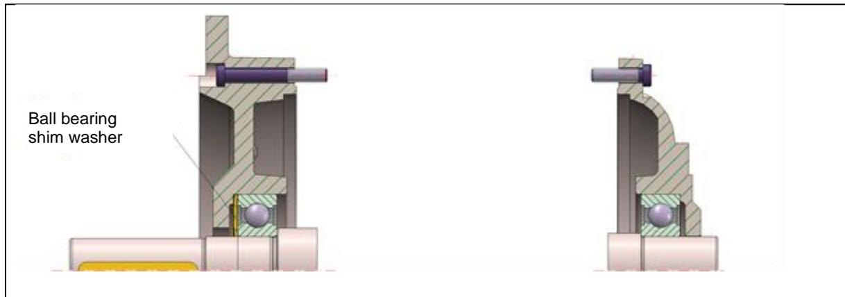
Fig. 1: Constructional design of bearings sizes 63-112
