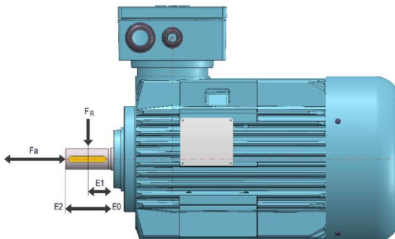
The nominal load of the bearings has been calculated for a minimum service life of 20 000 hours at a frequency of 50 Hz. Only axial loads are considered. The service life of the bearings is shorter when a combination of axial and radial loads is present.
