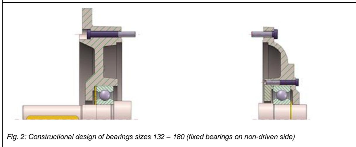
Fig. 2: Constructional design of bearings sizes 132 – 180 (fixed bearings on non-driven side)
