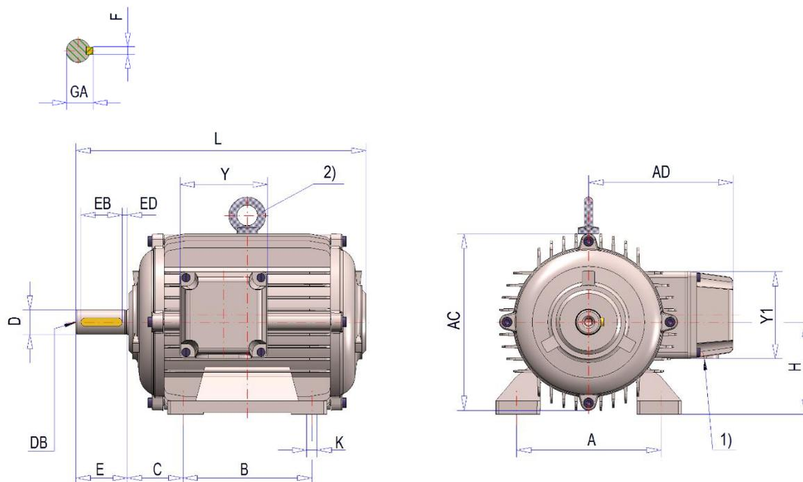
1) See planning section (Section *Cable glands in the terminal box*) Fits and tolerances see (Section *Fits and tolerances*)
