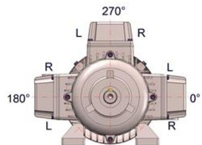
As standard, the brake release lever (if present) and the terminal box for the external fan are in line with the terminal box of the motor. Other versions must be ordered separately.
