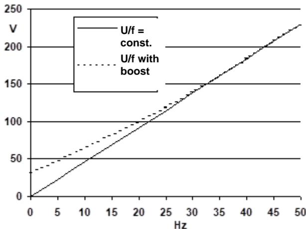
The illustration shows the  $U/f$  curves with and without boost. The frequency inverter makes determines the possible boost settings. The maximum torque of reluctance motors is proportional to the square of the voltage. As the ratio of the pull-out torque to the nominal torque is approximately 1.6 operation in the field weakening range ( $U = \text{constant}$ ) is not feasible or is only possible with limitations.
